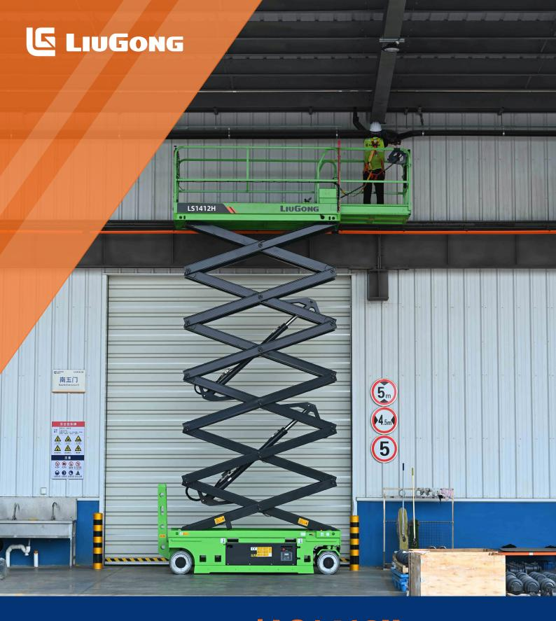
Working Height Max. 15.7 / 8 m (51'6" / 26'3")Overall Lift Capacity Max. 250 kg (551lb)Overall Width 1.25 m (4'1")Overall Length 2.84 m (9'4")Overall Weight 3,280 kg (7,231lb)
